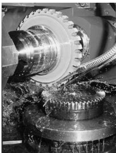
CNC machining of a PowerTRUE right-angle gear
