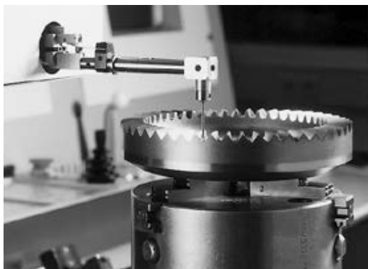
Computerized mapping of gear tooth profile
